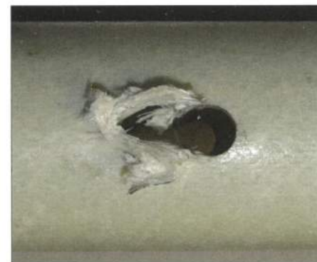
Fig. 15: Local bearing failure due to pin pressure
