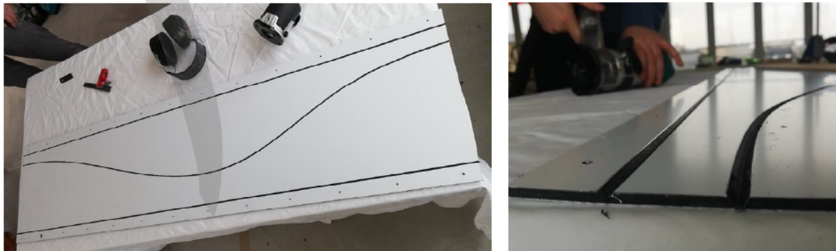
Fig. 12 Machining of the composite sheet to generate both straight and curved folds.
