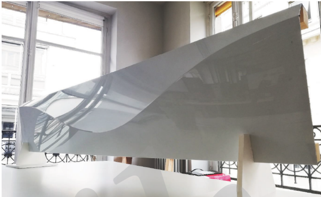
Fig. 13 Pictures of the prototype. The finish is very smooth and the reflections highlight the double-curved of the panel.
